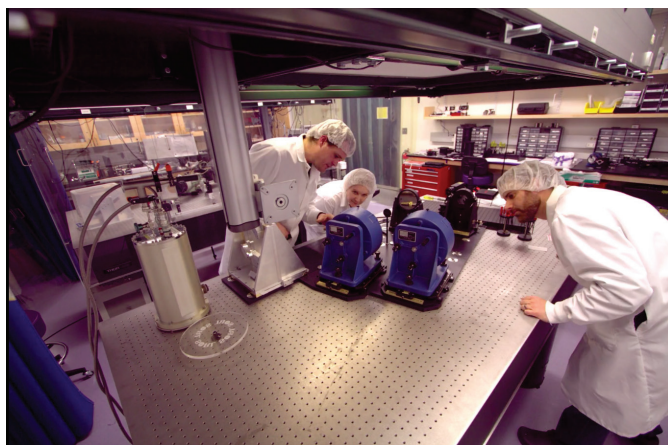
Screenshot from a time-lapsed video of the Exoplanets team assembling the MAO spectrometer. Courtesy of Yale Astronomy Department and Build Pictures.
